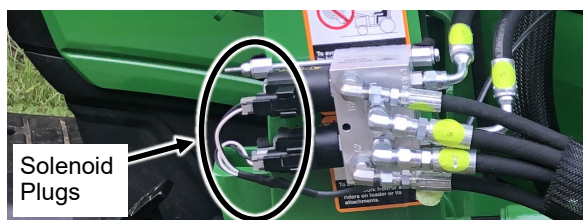
Fig. 4 (Attach Wire Harness Plugs to Solenoids)
